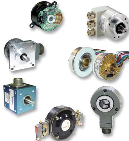
Encoder makers offer several types of discs that generate as many as two million counts per revolution and algorithms that decode them for extremely high resolution positioning. Encoders typically come with multiple channels, such as A and B, and their compliments to wash out any noise pulses that might contaminate the signal. Other signals and their compliments provide a reference position marker for homing and commutation.
