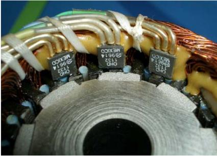
Hall-effect devices are digital On/Off sensors used to sense the presence of magnetic fields.
