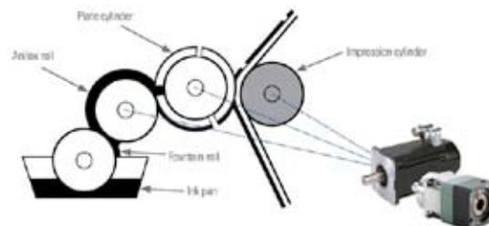
Figure 2 - In a “gearless” press configuration, each roller is driven independently by a motor/gearbox combination.
