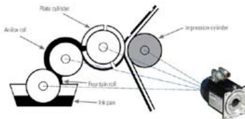
*Figure 3 - In a direct drive press configuration, all rollers are driven independently by a direct drive rotary motor, without the need for gears or gearboxes.*
