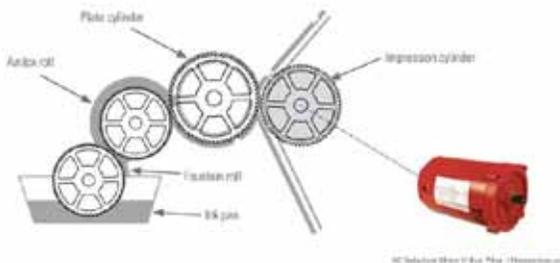
Figure 1 - In a geared press configuration, all rollers are tied together with gears driven by a single motor.
